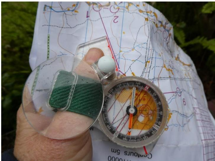
In the photo here you can see that the edge of my thumb compass is on the line of travel from the start to control 1 and I have rotated myself so that the north needle is parallel to the north lines on the map. (facing back toward me)
